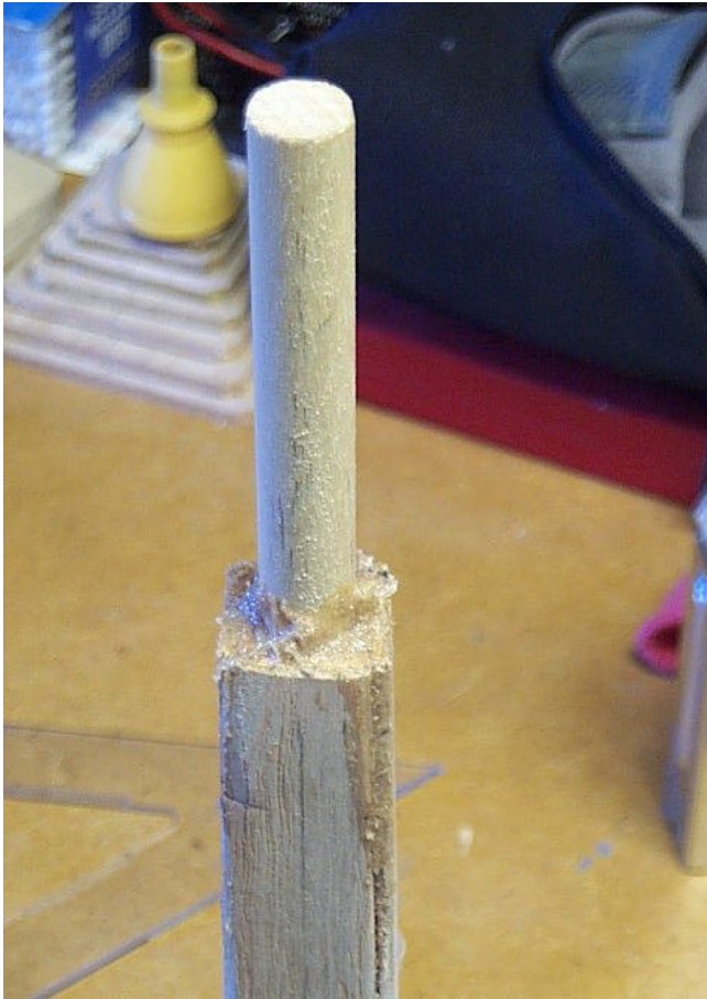
1/2" dowel epoxy-ed inside Bocal-A
