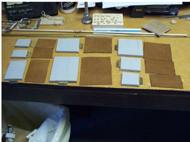
all keys with foam attached, ready for leather pads
