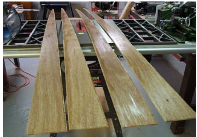
four trapezoids for Main section after varnishing
