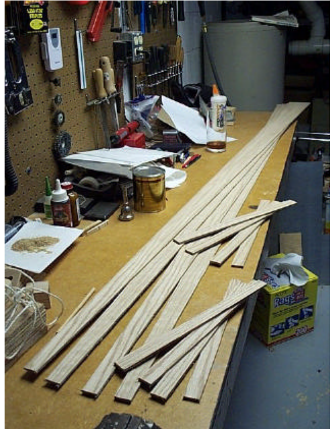
12 trapezoids after cutting from plywood sheet
