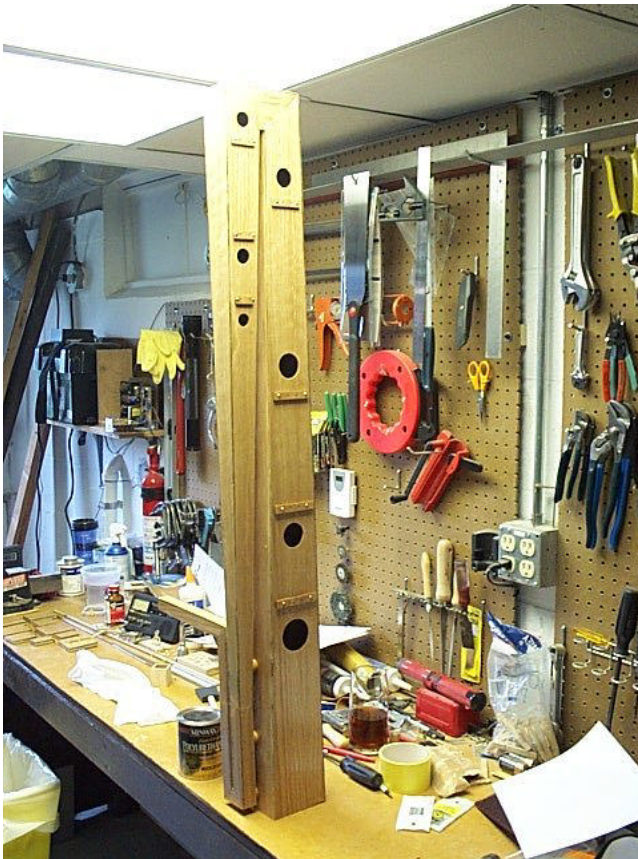
varnished BOC body, hinge blocks mounted & ready for keys - Note that this photo shows the hinge block for hole #2 in its original orientation; it was later moved perpendicular to the bore centerline and mounted to the side of the 'Up Tube'
