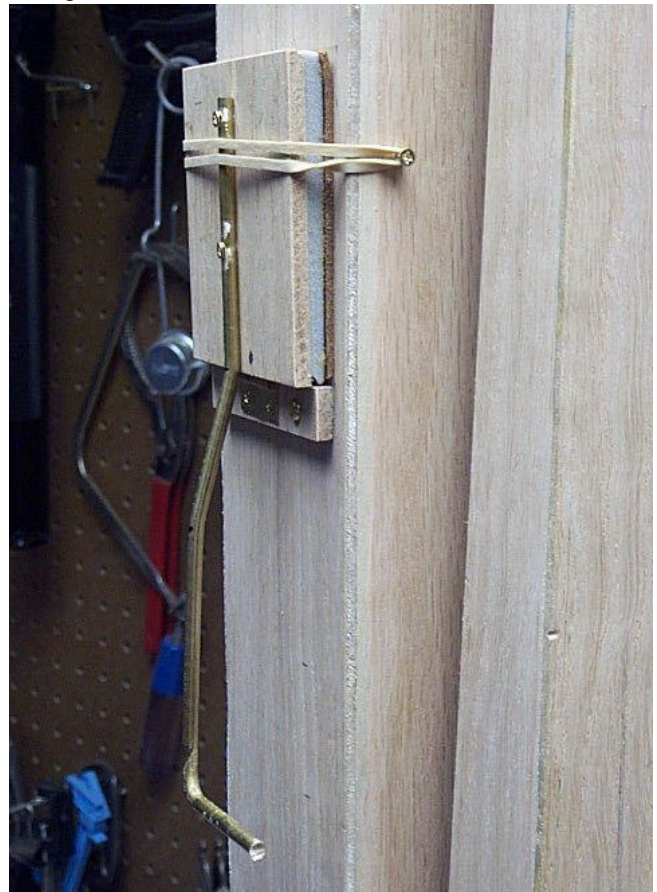
typical key lever, showing its mounting to the key
