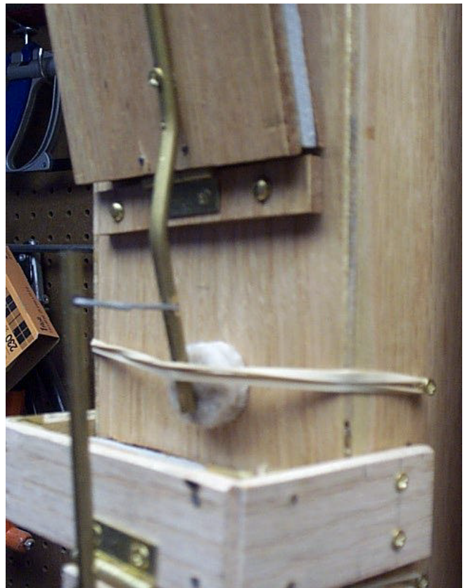
detail of key #9 lever pads and articulation
