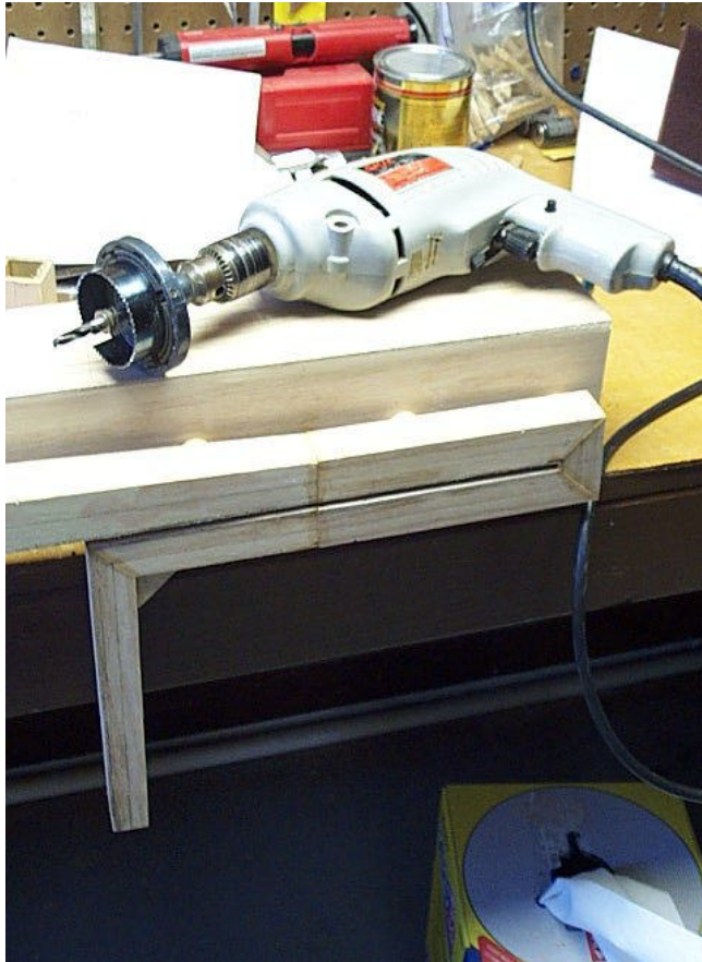
typical hole saw bit in electric drill
