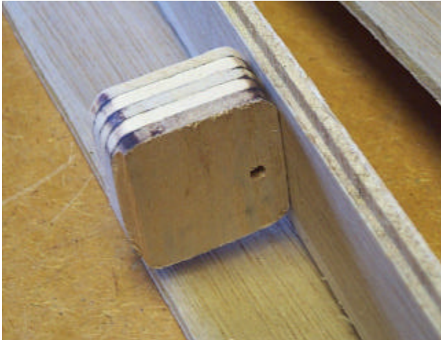
typical inner jig (hole should actually be centered)
